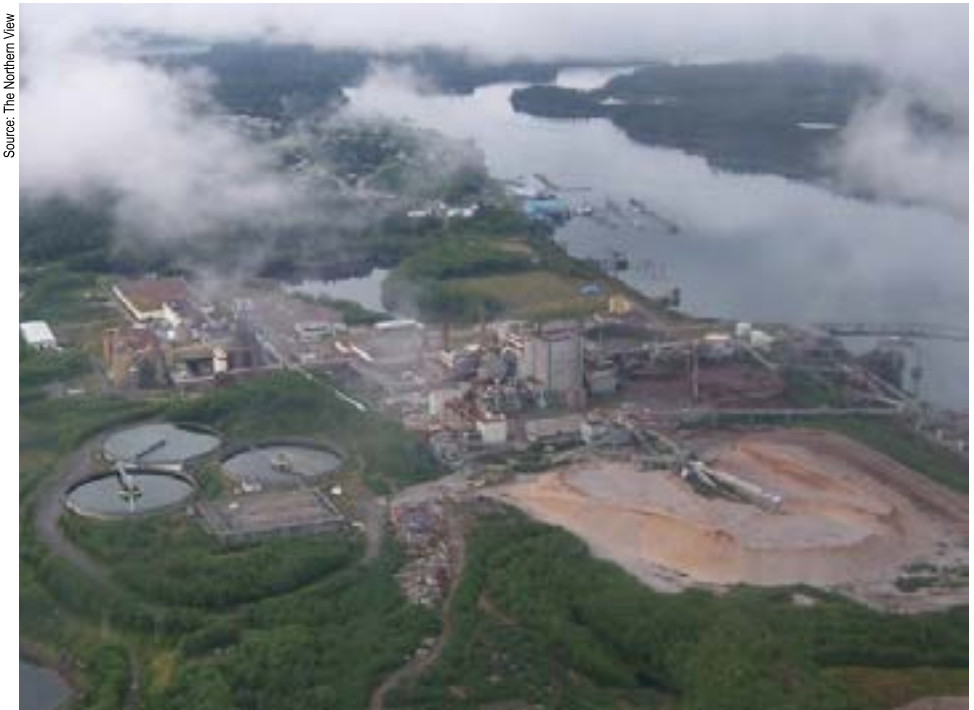
(fig.3) The Skeena Cellulose pulp mill. Clearly visible from an aerial view are potential environmental hazards including large lagoons, landfills, and an active railyard.
